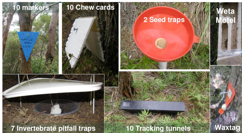
Figure A3.1. Monitoring devices deployed on each 450m monitoring line. In addition, one DoC automatic bird recorder is deployed per site (not shown).
